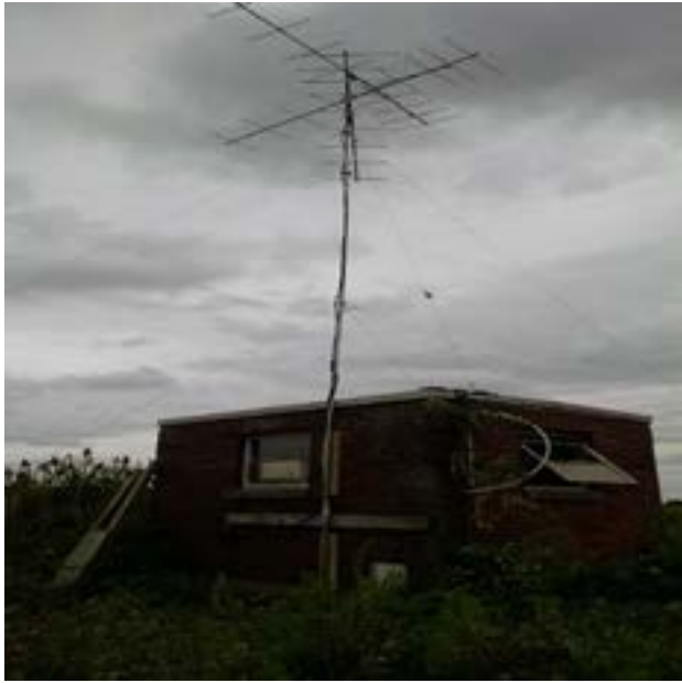
Photo by Chris Elphick Antenna array attached to nanotag receiver at Hammonasset Beach State Park.
